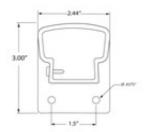
This Top Post End Bracket is made of cast aluminum and is in a dark bronze painted finish. It is designed to mount towards the top of our 9000/36/F and 9000/42/F receiver posts and will hold the top rails of our level picket rail panels 3642L.
