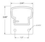
This Top Post End Bracket is made of cast aluminum and is in a black painted finish. It is designed to mount towards the top of our 9000/36/F and 9000/42/F receiver posts and will hold the top rails of our level picket rail panels 3642L.
