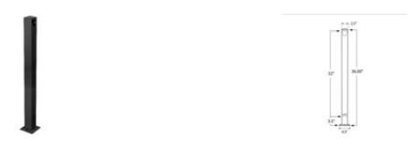
This 36" High Floor Mount End Post is a 2-1/2" square aluminum post that has two machined holes that are designed to receive the top and bottom rails of one picket rail panel. This post has a black paint finish.
