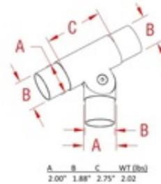
A streamlined look is achieved with the use of flush fittings. Different options ensure simple assembly and flexibility to accommodate any project. Our flush fittings feature a 1" long sleeve (The longest in the industry) for added strength and adhesive coverage.
