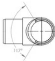
This elbow can connect to two different tubes.
