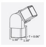
The Adjustable Flush Elbow for square tube is available in stainless steel and is designed to enable the connection of two equal tubes at various angles.
