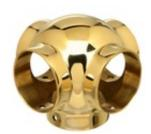
Ball fittings are used to construct handrails, footrails, stair rails, bar rails, ballet rails, and many other metal railing systems. The vertical posts of the railings should be made with a continuous architectural metal tube (for strength) while the horizontals are cut and fit with architectural hardware between posts. Ball fittings may be available in a variety of finishes not usually found in traditional brass fittings, including white, stainless steel, and more.
