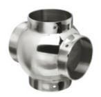
Ball fittings are used to construct handrails, footrails, stair rails, bar rails, ballet rails, and many other metal railing systems. The vertical posts of the railings should be made with a continuous architectural metal tube (for strength) while the horizontals are cut and fit with architectural hardware between posts. Ball fittings may be available in a variety of finishes not usually found in traditional brass fittings, including white, stainless steel, and more.
