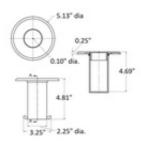
The 545 floor socket with cap is the fitting to use for removable railing and queueing posts. It is designed to hold 2" round tube and has a receiving space that is just over 2" in inside diameter to receive the tube. It is available in brass and 304 grade stainless steel and is mounted into the ground - typically core drilled into concrete. This item includes a cap to close the opening when there is no post in place.
