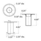
00-545/2 floor socket with cap is the fitting to use for removable railing and queueing posts. It is designed to hold 2" round tube and has a receiving space that is just over 2" in inside diameter to receive the tube. This item is made of brass with a polished finish on the top. and is mounted into the ground - typically core drilled into concrete. This item includes a cap to close the opening when there is no post in place.
