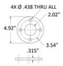
This floor mount flange is made of type 316 stainless steel, has a brushed finish on one side and is designed to hold 2" OD round tube. It has four thru holes for mounting hardware. Weld this flange to the stainless steel tube that fits into the center hole.
