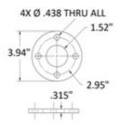
This floor mount flange is made of type 316 stainless steel, has a brushed finish on one side and is designed to hold 1-1/2" OD round tube. It has four thru holes for mounting hardware. Weld this flange to the stainless steel tube that fits into the center hole.
