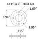
This floor mount flange is made of type 316 stainless steel, has a brushed finish on one side and is designed to hold 1.67" OD round tube. It has four thru holes for mounting hardware. Weld this flange to the stainless steel tube that fits into the center hole.
