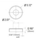
The 49-540/2 round flange canopy or escutcheon plate is made of 316 grade stainless steel, has a polished finish and allows for a 2" diameter round tube to pass through its center hole. Use this cover as a decorative addition to flanges that are often unseemly because of the mounting hardware used with them.
