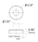
The 49-540/1H round flange canopy or escutcheon plate is made of 316 grade stainless steel, has a satin (brushed) finish and allows for a 1-1/2" diameter round tube to pass through its center hole. Use this cover as a decorative addition to flanges that are often unseemly because of the mounting hardware used with them.
