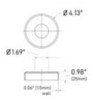
The 49-540/424 round flange canopy or escutcheon plate is made of 316 grade stainless steel, has a satin (brushed) finish and allows for a 1.67" diameter round tube to pass through its center hole. Use this cover as a decorative addition to flanges that are often unseemly because of the mounting hardware used with them.
