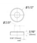
The 47-540/2 round flange canopy or escutcheon plate is made of 316 grade stainless steel, has a polished finish and allows for a 2" diameter round tube to pass through its center hole. Use this cover as a decorative addition to flanges that are often unseemly because of the mounting hardware used with them.
