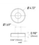
The 47-540/424 round flange canopy or escutcheon plate is made of 316 grade stainless steel, has a polished finish and allows for a 1.67" diameter round tube to pass through its center hole. Use this cover as a decorative addition to flanges that are often unseemly because of the mounting hardware used with them.
