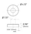
The 40-540/1H round flange canopy or escutcheon plate is made of 304 grade stainless steel, has a polished finish and allows for a 1-1/2" diameter round tube to pass through its center hole. Use this cover as a decorative addition to flanges that are often unseemly because of the mounting hardware used with them.
