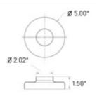
The 00-540/2 round flange canopy or escutcheon plate is made of brass, has a polished finish and allows for a 2" diameter round tube to pass through its center hole. Use this cover as a decorative addition to flanges that are often unseemly because of the mounting hardware used with them.
