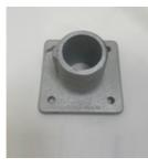
The Speed-Rail® Square Base Flange is made of cast aluminum-magnesium alloy 535 and is available for pipe 1-1/2".
