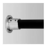
Item 28106 is made of aluminum-magnesium alloy 535 and includes two screws to hold the pipe in place. It is designed to hold 1-1/2" IPS pipe (see item A112ID) and has an anodized finish.
