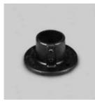
Item 55BK-28090 is made of aluminum-magnesium alloy 535, has a matte black powder coat finish, and includes two screws to hold the pipe in place. It is designed to hold 1-1/2" IPS pipe (see item A112ID).
