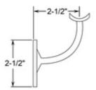
This wall mount handrail bracket is made of 316 stainless steel, has a brushed (satin) finish and is designed to hold 1-1/2" outside diameter round tube. The back plate has three counter sunk holes that can be positioned for horizontal or angled handrail. Mount this bracket on a wall (recommended on a stud) or on a rectangular vertical post using the included hardware or alternate depending on the material the bracket is being mounted upon.
