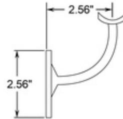
This wall mount handrail bracket is made of 316 stainless steel, has a brushed (satin) finish and is designed to hold 1.67" outside diameter round tube. The back plate has three counter sunk holes that can be positioned for horizontal or angled handrail. Mount this bracket on a wall (recommended on a stud) or on a rectangular vertical post using the included hardware or alternate depending on the material the bracket is being mounted upon.
