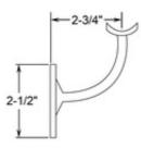
This wall mount handrail bracket is made of 316 stainless steel, has a polished finish and is designed to hold 2" outside diameter round tube. The back plate has three counter sunk holes that can be positioned for horizontal or angled handrail. Mount this bracket on a wall (recommended on a stud) or on a rectangular vertical post using the included hardware or alternate depending on the material the bracket is being mounted upon.
