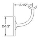
This wall mount handrail bracket is made of 316 stainless steel, has a polished finish and is designed to hold 1-1/2" outside diameter round tube. The back plate has three counter sunk holes that can be positioned for horizontal or angled handrail. Mount this bracket on a wall (recommended on a stud) or on a rectangular vertical post using the included hardware or alternate depending on the material the bracket is being mounted upon.
