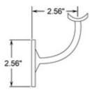
This wall mount handrail bracket is made of 316 stainless steel, has a polished finish and is designed to hold 1.67" outside diameter round tube. The back plate has three counter sunk holes that can be positioned for horizontal or angled handrail. Mount this bracket on a wall (recommended on a stud) or on a rectangular vertical post using the included hardware or alternate depending on the material the bracket is being mounted upon.
