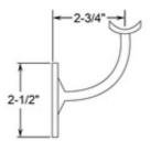
This wall mount handrail bracket is made of 304 grade stainless steel, has a polished finish and is designed to hold 2" outside diameter round tube. The back plate has three counter sunk holes that can be positioned for horizontal or angled handrail. Mount this bracket on a wall (recommended on a stud) or on a rectangular vertical post using the included hardware or alternate depending on the material the bracket is being mounted upon.
