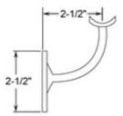
This wall mount handrail bracket is made of 304 grade stainless steel, has a polished finish and is designed to hold 1-1/2" outside diameter round tube. The back plate has three counter sunk holes that can be positioned for horizontal or angled handrail. Mount this bracket on a wall (recommended on a stud) or on a rectangular vertical post using the included hardware or alternate depending on the material the bracket is being mounted upon.
