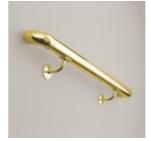
This Wall mount handrail bracket is made of brass, has a polished finish and is designed to hold 2" outside diameter round tube. The back plate has three counter sunk holes that can be positioned for horizontal or angled handrail. Mount this bracket on a wall (recommended on a stud) or on a rectangular vertical post using the included hardware or alternate depending on the material the bracket is being mounted upon.
