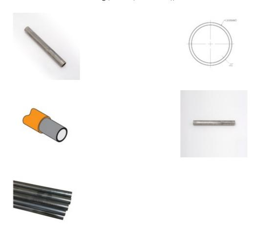
The 20-A120SL steel insert has a 1-7/8" outside diameter and fits inside 2"  $\times$  0.05" wall architectural tube. The insert serves to reinforce the tube and is available in 12 foot stock lengths.
