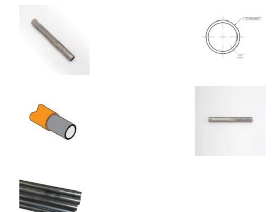
The 20-A100SL steel insert has a 7/8" outside diameter and fits inside 1" x 0.05" wall architectural tube. The insert serves to reinforce the tube and is available in 12 foot stock lengths.
