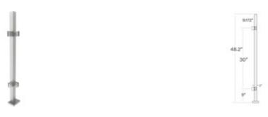
The 48" high floor mount partition post is made of 2" square tube and 316 grade satin (brushed) stainless steel. This corner post comes with a CUT flange welded at the bottom, a flange canopy, four glass grips attached to the post and a flush end cap on the top.
