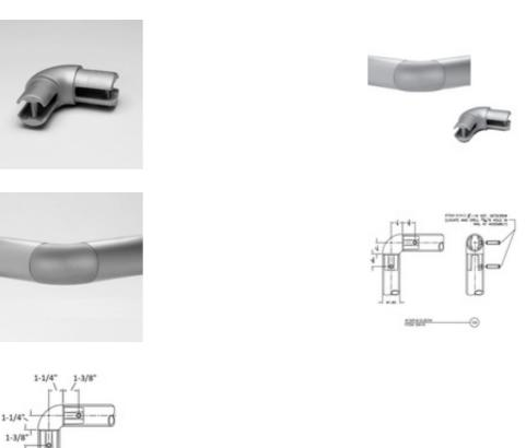
Interna-Rail® item# 58016 is a cast aluminum 90 degree elbow with an anodized finish and is designed to connect with 1-1/2" IPS schedule 40 pipe. This item includes two set screws that are used to connect the pipe to the fitting.
